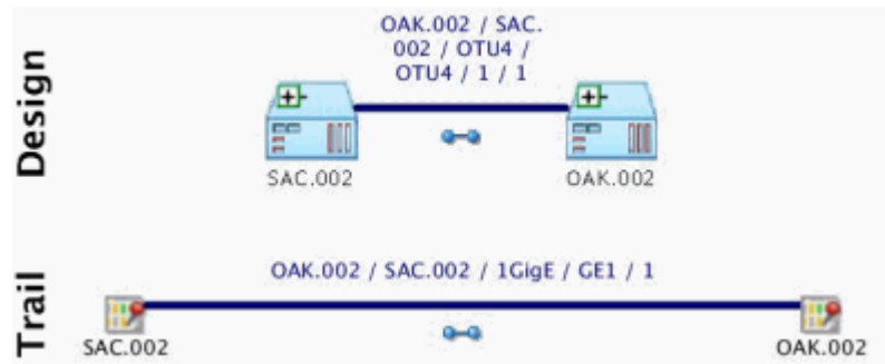
Figure 14-14 Schematic View of 1GigE Connectivity Enabled by OTN Connectivity
