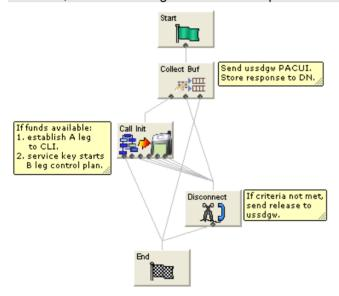
The Call Initiation node will start a simple control plan which connects the A leg based on the CLI. A second control plan is started when the A leg answers and a new IDP arrives at slee\_acs with the service key from the Call Initiation node. The second control plan connects the B leg normally (for example by using an Attempt Terminate node).
