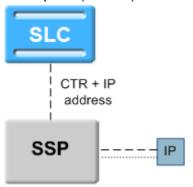
The SLC communicates with the SSP through the ETC (EstablishTemporaryConnection) and IP address. The SSP then uses the IP address to communicate with an external IP.
