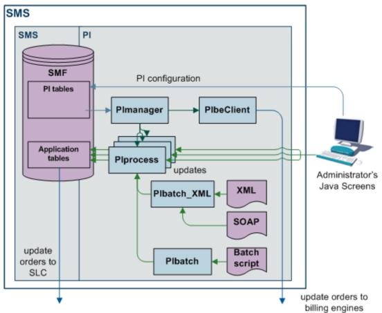
This diagram shows the PI components and processes.
