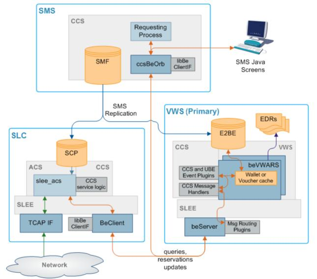
Here is an example of how the VWS handles requests from CCS on an SLC to a VWS.
