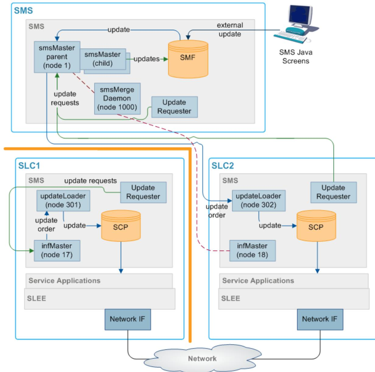
Where an SLC has been isolated from the master it looks for and connects to the master in the network, which has the next lowest node number. In the diagram above, SLC1 has been isolated from the network and the update loader cannot find Master 1, so it looks for the master with the lowest node number it can see (in this case it is Inferior Master 2 on SLC1) and connects to that.
