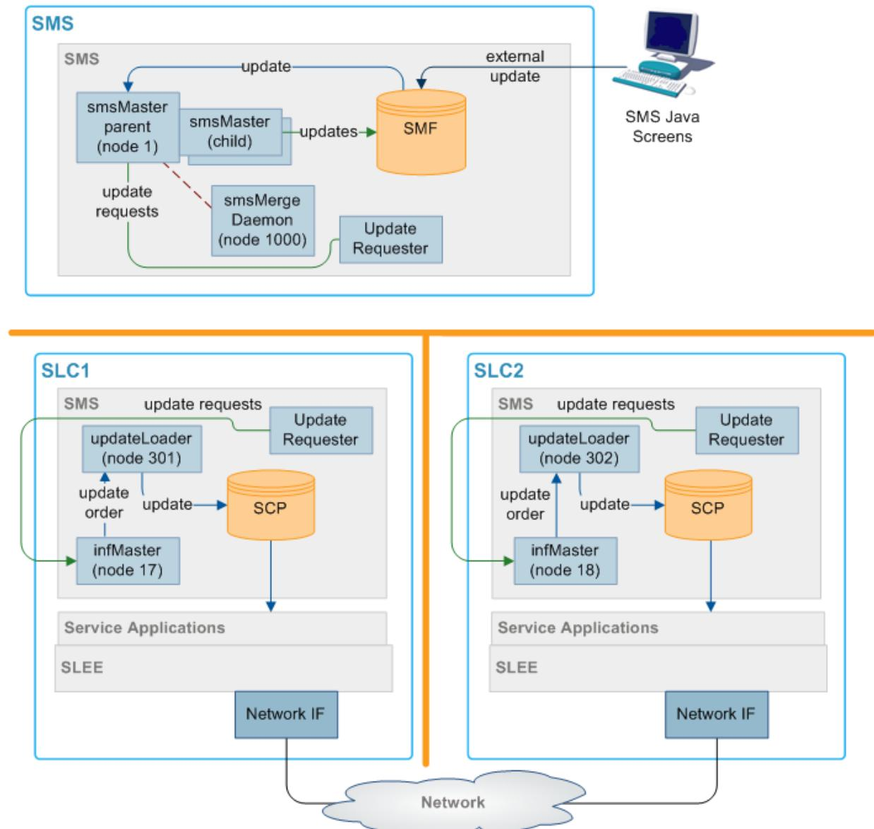
Where all nodes in the network are isolated, they each connect to the inferior master with the lowest node number that they can see. In the above example, this results in the update loader on SLC1 connecting to inferior master 2 on SLC1 (node 2), and the update loader on SLC2 connecting to the inferior master 3 (node 3).
