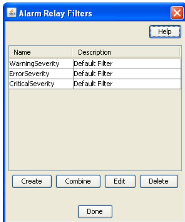
**Note:** This screen is accessed through the **Edit Filters** button on the alarm **Notification** tab.
