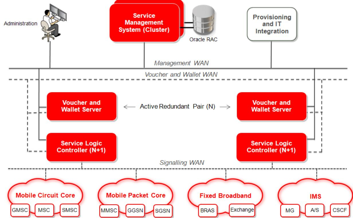
**Note:** The configuration of the VWS in a redundant pair set-up and the SLC running in an N+1 configuration. Here the SMS is set up in a redundant cluster configuration using Oracle RAC for the database component.
