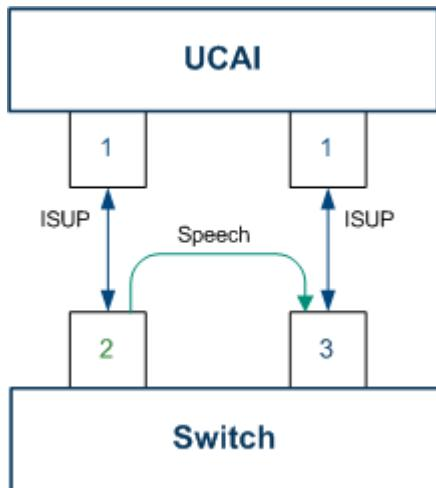
**Note:** The major difference between this and the 'per link' fix is there are now two signalling links involved. The signalling for the traffic from the switch to the UCAI uses one link, while the signalling for the traffic coming from the UCAI to the switch uses the other.
