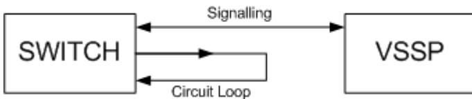
As shown in the example, the only actual connection to UCAI is the signaling link. No speech paths are routed. All signaling, for both the incoming and outgoing circuits on the loop, are carried on the signaling link. The speech path is looped with very low visibility to the switch. This may be achieved by using a static configuration of the switch matrix, or by an external piece of hardware. In either case, the switch's call process is unaware of the loop.
