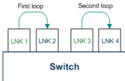
Quite how the signalling would work in this situation is somewhat unclear. However, it is possible to do it with just the one signalling link, provided care is taken to assign the cics correctly.
