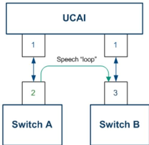
In this case, UCAI is simply modifying the signalling on an otherwise ordinary link between two switches. The timeslots associated with link management and speech (usually, all except 16) are left intact. UCAI takes the signalling out to be processed.
