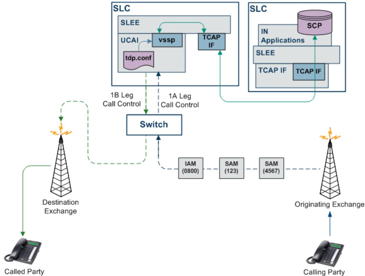
The originating exchange will attempt to set up a call once it has collected sufficient digits from the calling party to identify the next target exchange (tandem or ultimate destination exchange) in the call flow. It will generate an IAM (Initial Address Message) with all the digits the calling party has dialed until then, and route it along the network.
