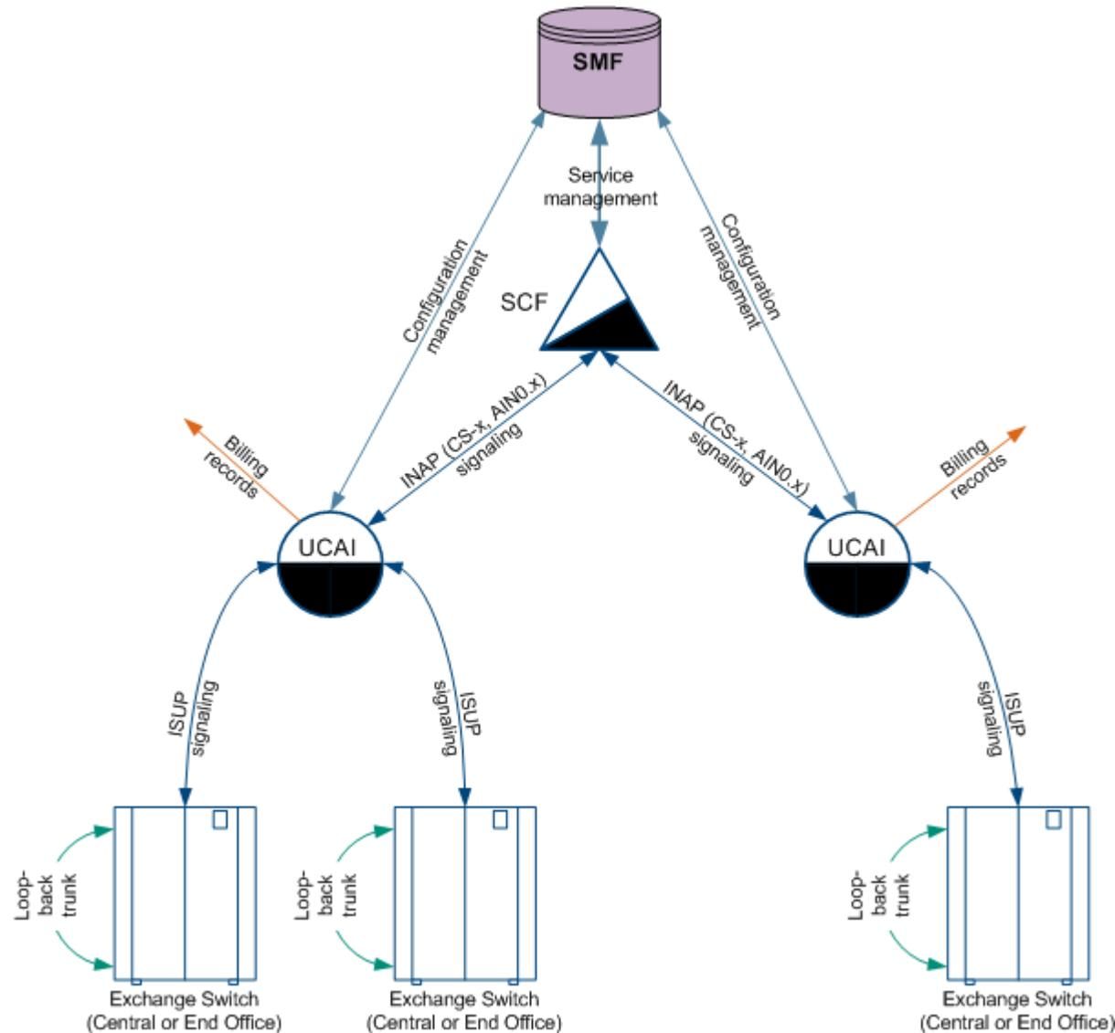
**Note:** Although the UCAI is shown as a separate physical entity in this diagram, it may also co-exist on the SLCs. If so, it will still communicate with the SCF over INAP (though this may not leave the SS7 stack).
