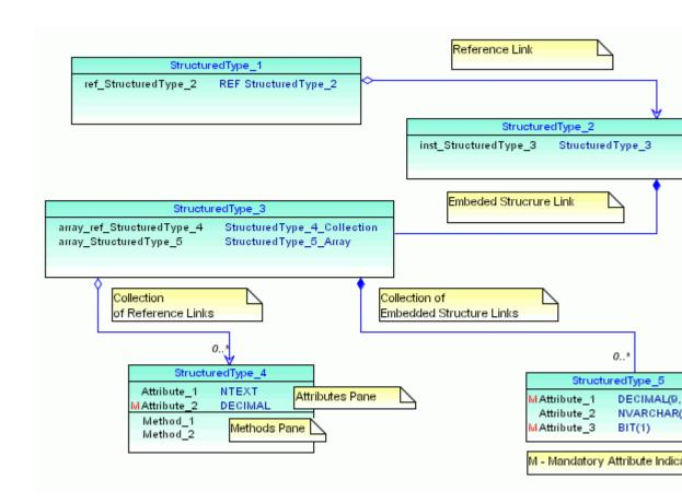
A structured type box contains the name of the object, its defined attributes, and its methods (if any). Diagram links represent various kinds of attributes with a structured data type.
