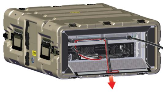
**c.** Connect the power cable into the port located in right cable channel, route cable slack through the foam channel and cable mount, and through the oval cutout on the EMI Filter assembly as shown.
