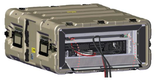
**Tighten the Rear EMI Filter Assembly Captive Screws**
