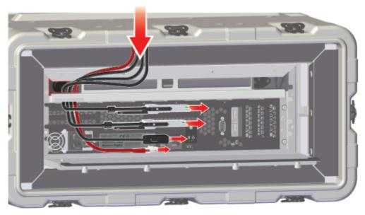
**b.** Connect each cable into the designated ports, route cable slack through the foam channels, and route the other end of the data cables through the oval cutout on the EMI Filter assembly.
