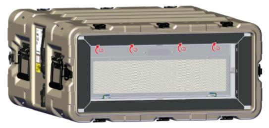
c. Be aware and ensure that the ground cables on the EMI Filter assembly do not get pinched during reinstallation.
