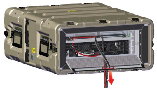
**d.** With the cables secured in place rotate and push the EMI Filter assembly forward to align the captive screws with the screw holes and begin tightening them with thumb and finger. Be sure to apply pressure as the foam channels that route cables will provide resistance. Once the cables and EMI filter are properly in place, use a T15 Torx screwdriver to tighten the captive screws on the front EMI Filter assembly.
