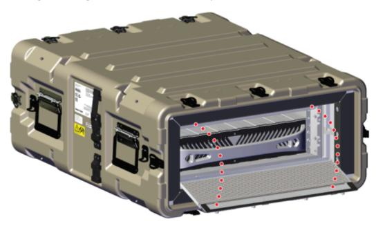
b. Use a T15 Torx screwdriver to tighten the captive screws on the front EMI Filter assembly.
