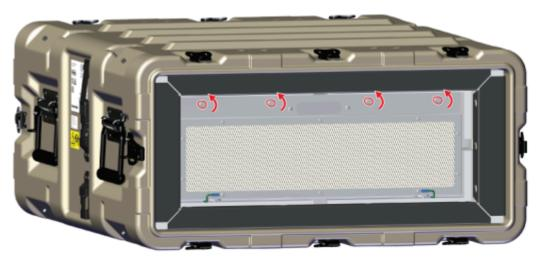
**b.** Carefully rotate the top of the EMI filter assembly down until it is resting on the case as shown in the following image.
