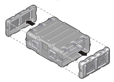
**4.** Remove the cable pouch, and extend the end-cap hooks.
