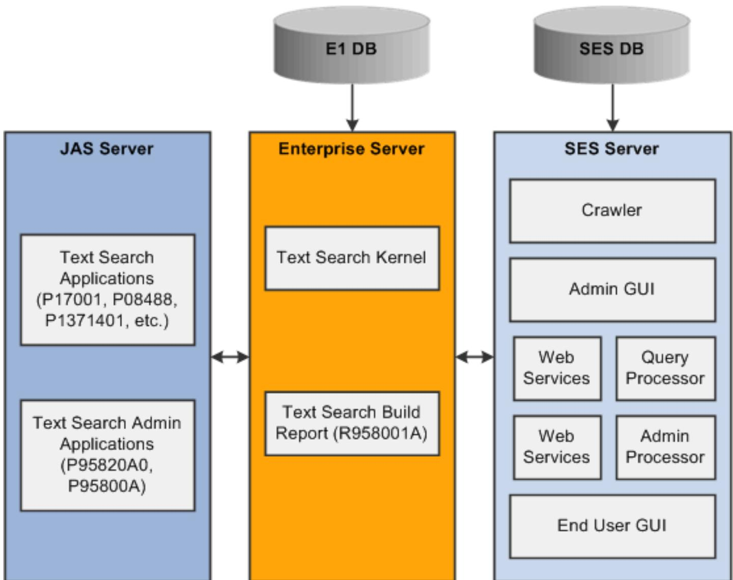
Records from text enabled business views are fed into the SES server to index in the form of XML feeds. SES server reads these XML feeds and indexes them under the source group created in the name of business view/data source combination.
