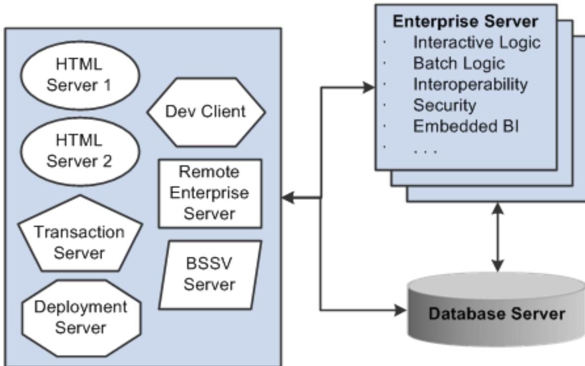
The Enterprise Server is the central hub that receives requests from multiple clients as well as other Enterprise Server Instances. It communicates with the database for transactional processing and can be clustered for failover and hot-swap capabilities.
