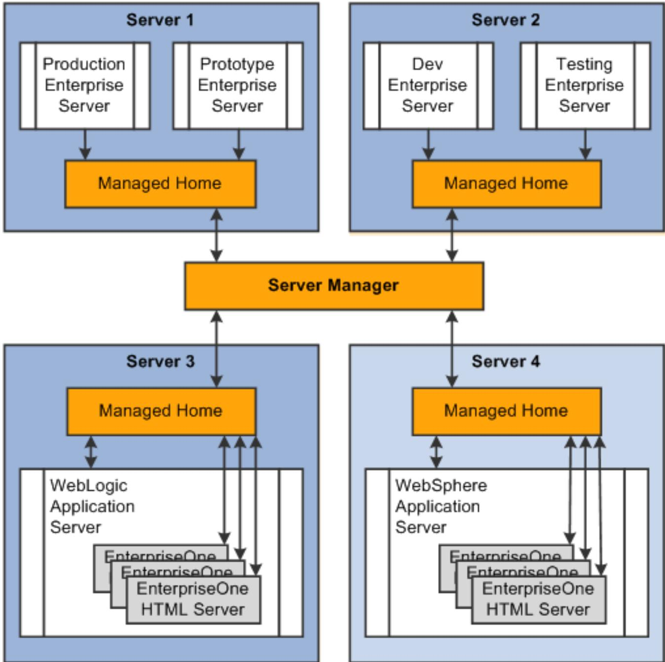
Server Manager consists of a web based 'console' application and a set of 'agents' that communicate with the console. The console sends control commands and information requests to the agents and the agents pass along control commands to the local web application server or enterprise server or reports status and runtime information back to the console.
