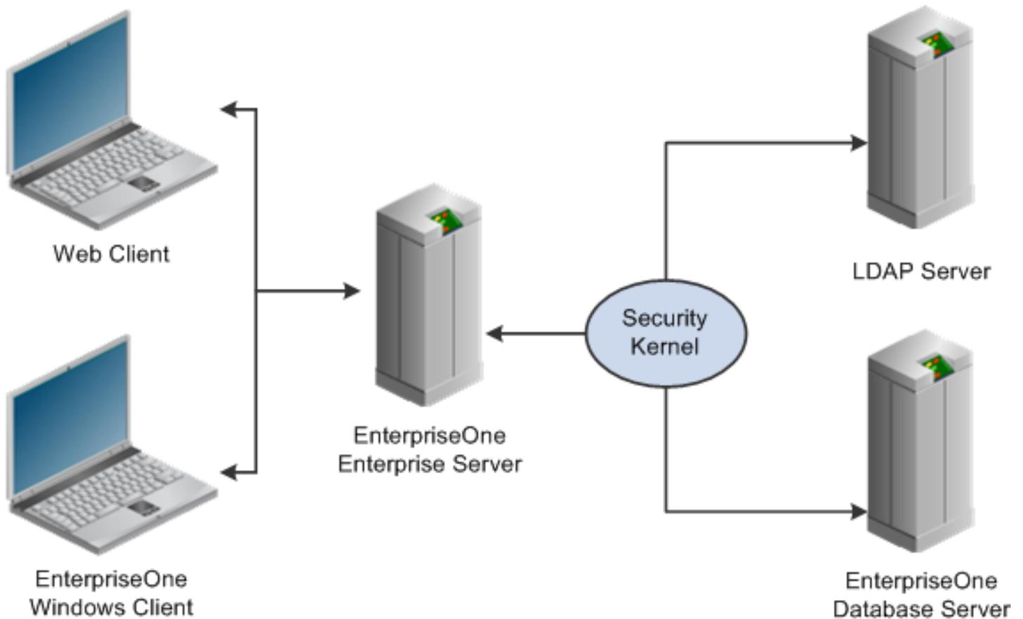
The security kernel in the Enterprise Server performs authentication against the LDAP server when LDAP is enabled in the [SECURITY] section of the jde.ini file of the Enterprise Server. Otherwise, when LDAP is disabled, the security kernel authenticates the user against the Enterprise Server database.
