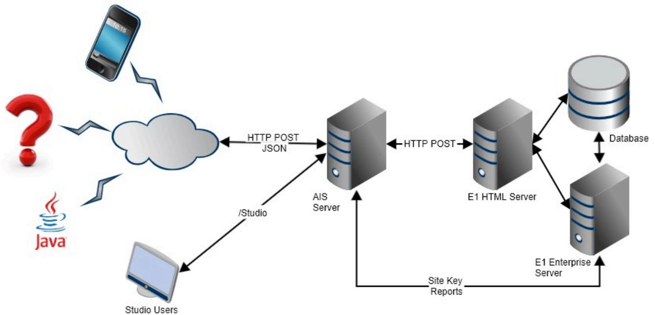
**Note:** The Orchestrator Studio 9.2.4 is deployed along with the AIS server 9.2.4.0 and can be accessed by using the AIS Server URL. Therefore, the Orchestrator Studio 9.2.4 does not require any additional set-up or installation steps. The JD Edwards EnterpriseOne Orchestrator Studio 9.2.4 is installed on AIS server instance. (Release 9.2.4.0)
