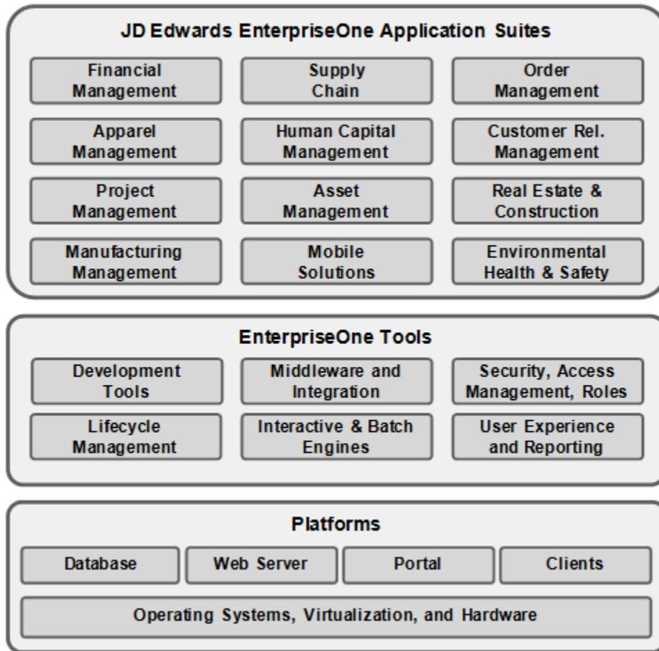
The following illustration provides a high-level overview of the components that comprise the JD Edwards EnterpriseOne technology layer. These components enable functionality such as user interface, security, reporting, and so on, across all JD Edwards EnterpriseOne application modules. Although depicted and often named as servers, these are actually logical components, which often can be colocated on the same physical hardware or installed into virtual machines.
