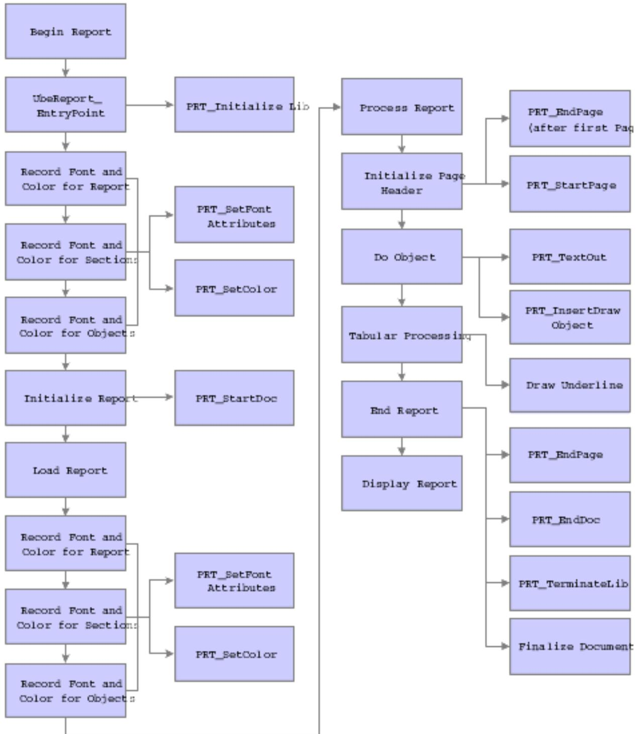
At each of these execution points, with the exception of PRT\_InitializeLib and PRT\_TerminateLib, you can call an OSA function. You can create functions or you can use existing XML libraries and their functions.
