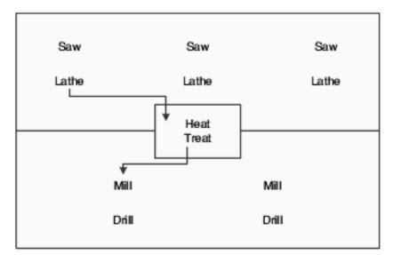
After you have defined the item's bill of material and where each operation occurs on the factory floor (work center), you must define the sequence of operations that is necessary to manufacture the item (routing instructions).
