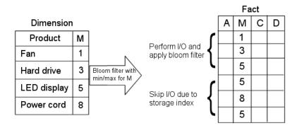
The I/O for the second block of the fact table is completely eliminated by Storage Indexes as its minimum/maximum range (5,8) is not present in the Bloom filter.
