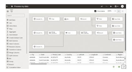
To build a data flow, you add steps. Each step performs a specific function, for example, add data, join tables, merge columns, transform data, save your data. Use the data flow editor to add and configure your steps. Each step is validated when you add or change it. When you've configured your data flow, you execute it to produce or update a dataset.
