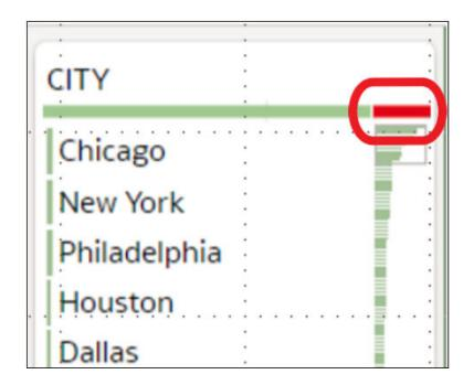
• **Replace or correct** - When you've identified anomalies and outliers, use inline replace to correct values. You get immediate feedback on the improvements to the data quality on the quality bar.
