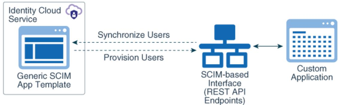
In this diagram, the Generic SCIM App Template has been configured to enable Oracle Identity Cloud Service to communicate with a custom application that has a SCIM-based interface. This interface uses REST API endpoints to provision and synchronize users between Oracle Identity Cloud Service and the custom application.
