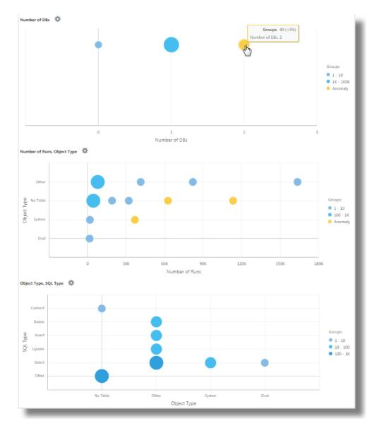
In the bubble charts, the log records are grouped based on the number of SQLs that fall under each set of parameters. The <code>Object Type</code> and <code>SQL Type</code> parameters are determined using the <code>eval</code> command in the query.
