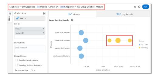
1. To create an alert rule that will notify you upon detecting anomalies, you must first define the condition in the query. Edit the highlighted query, and add the where command to define the Group Duration in which the anomalies are found, that is, when it's more than or equal to 60,000 milliseconds. For example:
