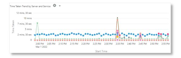
In the above example, the X-axis shows the values from the *Start Time* field. The Y-axis shows the time taken using the average of the numeric field *Duration* in seconds. Each series in the chart represents a unique combination of *Server* and *Service*.
