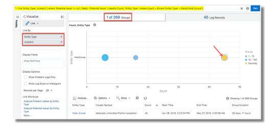
The groups table displays the details of the cluster sample corresponding to the anomaly group. Note the log content of the cluster sample available in the table which is possibly the cause for the potential issue: detected unhandled Python exception.
