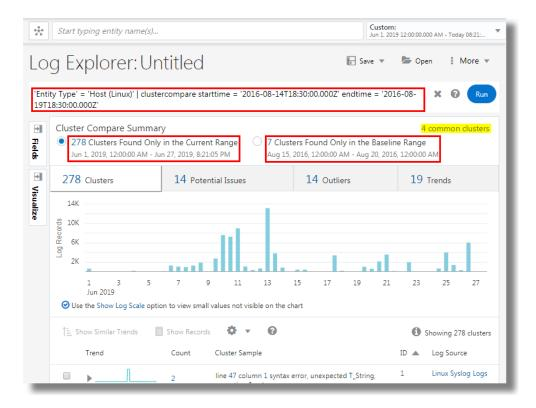
This analysis can enable you to compare the syslog data from the entity type over the two periods, eliminate the common clusters, and view the unique clusters. In this case, the increase in the number of potential issues from the baseline range to current time range can be analyzed by viewing the logs pertaining to the potential issues in the current time range.
