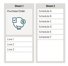
If, instead, the workbook uses a Table layout as the primary layout, then each level in the hierarchy has its own Table layout on a separate worksheet. In this diagram, Sheet 1 includes a Table layout for the parent business object showing the details for three purchase orders. Sheet 2 and Sheet 3 includes dependent Table layouts for the child and grandchild business objects, respectively.
