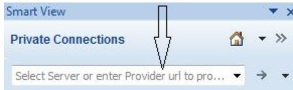
Figure 3-1 Text Box for Entering URL when Creating a Quick Connection
