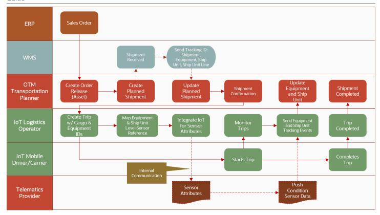
This section describes the functional flow of information between an order management ERP, OTM and IoT FM to monitor cargo conditions, equipment conditions and track equipment locations.
