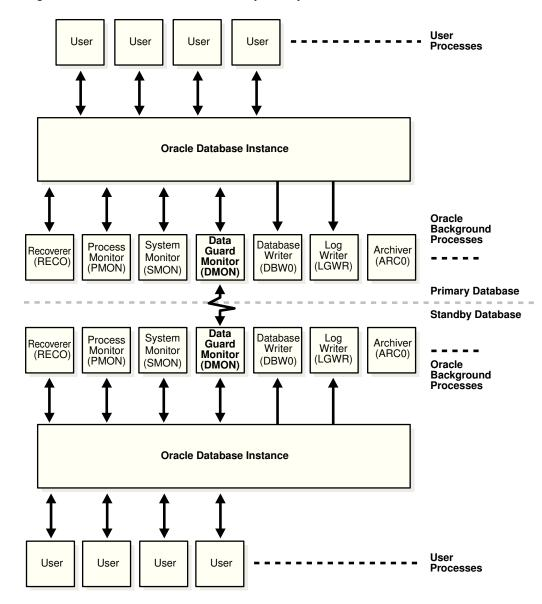
Figure 1-2 Databases With Broker (DMON) Processes
