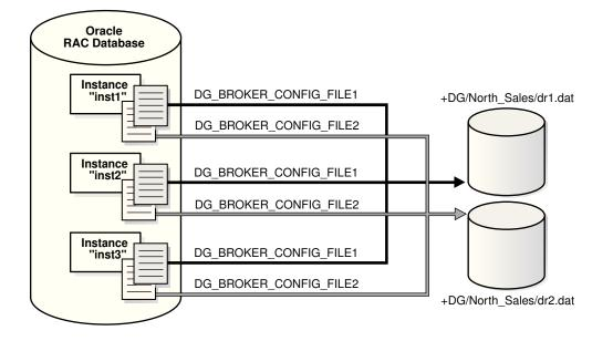
Figure 3-3 Broker Configuration Setup with Oracle ASM
