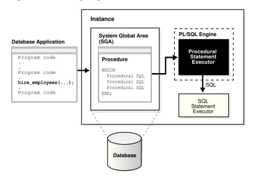
Figure 8-3 The PL/SQL Engine and Oracle Database
