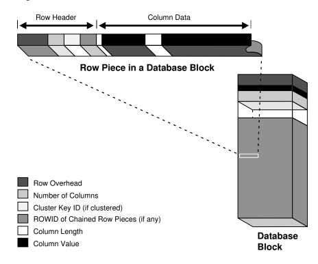
Figure 12-8 The Format of a Row Piece
