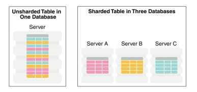
Figure 1-5 Horizontal Partitioning of a Table Across Shards
