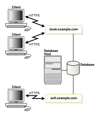
Figure 16-6 Multiple Services Associated with One Database
