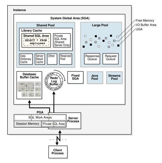
Figure 14-1 Oracle Database Memory Structures
