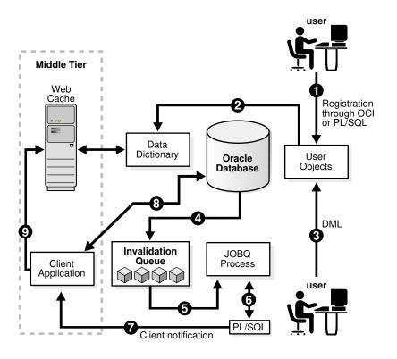
Figure 18-2 Basic Process of Continuous Query Notification (CQN)
