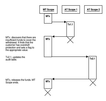
Figure 8-7 Bank Withdrawal—Insufficient Funds with Overdraft Protection
