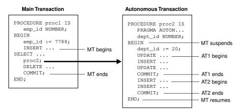
When you enter the executable section of an autonomous transaction, the main transaction suspends. When you exit the transaction, the main transaction resumes. COMMIT and ROLLBACK end the active autonomous transaction but do not exit the autonomous transaction. As Figure 8-3 shows, when one transaction ends, the next SQL statement begins another transaction.
