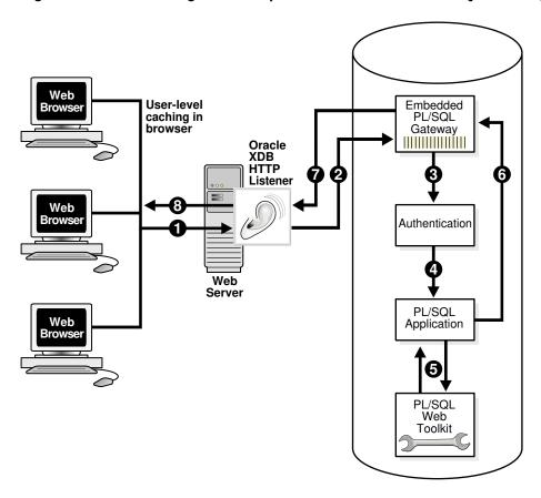
Figure 17-2 Processing Client Requests with Embedded PL/SQL Gateway
