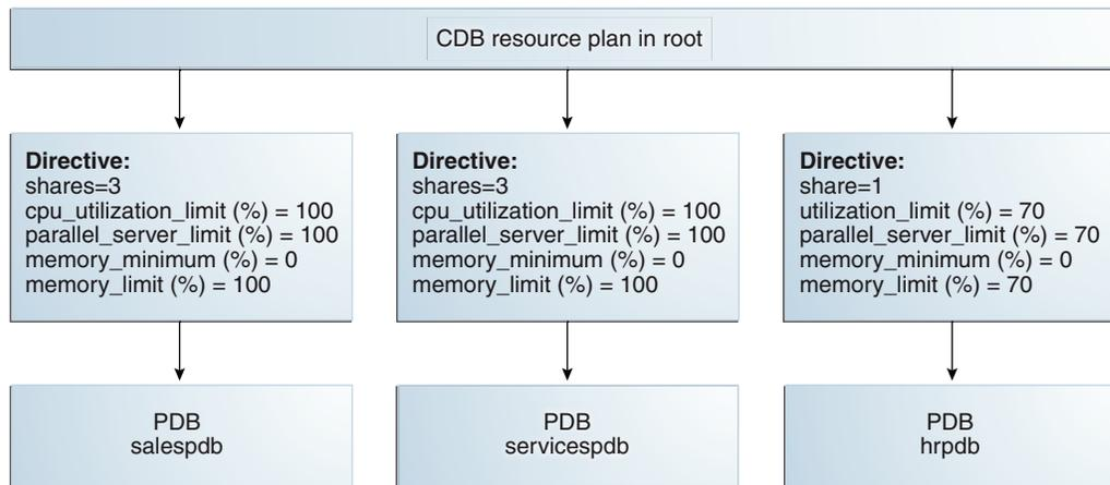
Figure 12-2 shows that there are no utilization limits on the salespdb and servicespdb PDBs because the `cpu_utilization_limit (%)` and `parallel_server_limit (%)` directives are both set to 100 for them. However, the hrpdb PDB is limited to 70% of the applicable system resources because the `cpu_utilization_limit (%)` and `parallel_server_limit (%)` directives are both set to 70.
