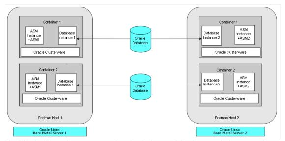
The following figure shows two examples of typical test and development deployments. The example on the left side shows a Podman host in which the cluster member nodes are containers in the same Podman host. The example on the right shows two Podman hosts on the same hardware server, with separate containers on each host.
