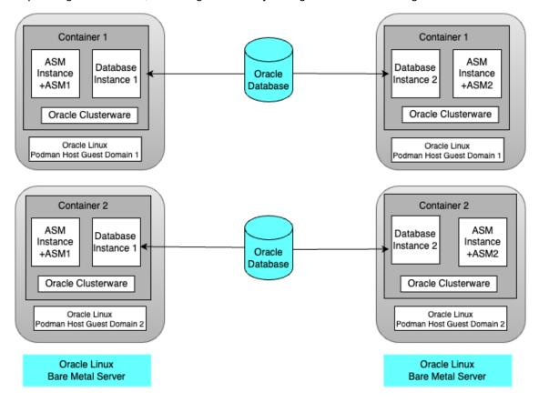
The following figure shows another production deployment, in which containers are located in different Podman hosts on separate hardware servers, with a high availability storage and network configuration:
