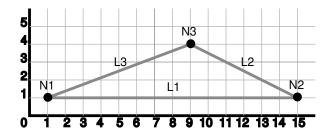
As shown in Figure 5-4, node N1 is at point 1,1, node N2 is at point 15,1, and node N3 is at point 9,4. Link L1 is a straight line connecting nodes N1 and N2, link L2 is a straight line connecting nodes N2 and N3, and link L3 is a straight line connecting nodes N3 and N1. There are no other nodes or shape points on any of the links.
