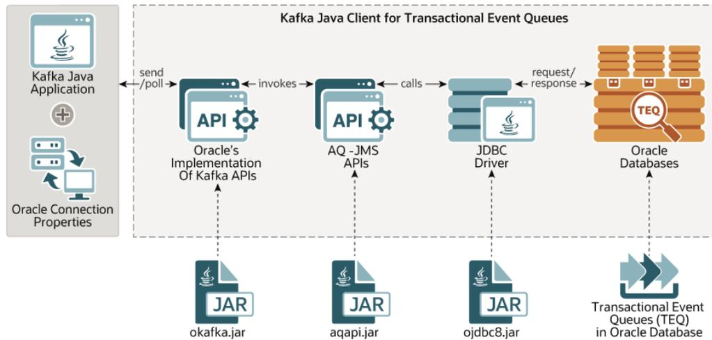
The figure shows OKafka library, which contains Oracle specific implementation of Kafka's Java APIs. This implmentation internally invokes AQ-JMS APIs which in turn uses JDBC driver to communicate with Oracle Database.
