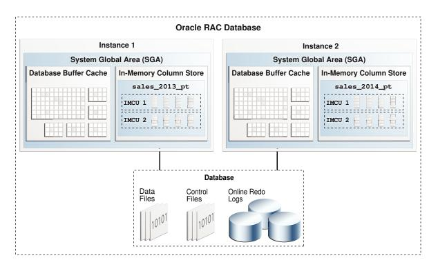
Figure 12-3 Automatic In-Memory Distribution in Oracle RAC
