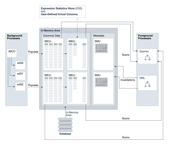
Figure 2-5 IM Column Store: Memory and Process Architecture
