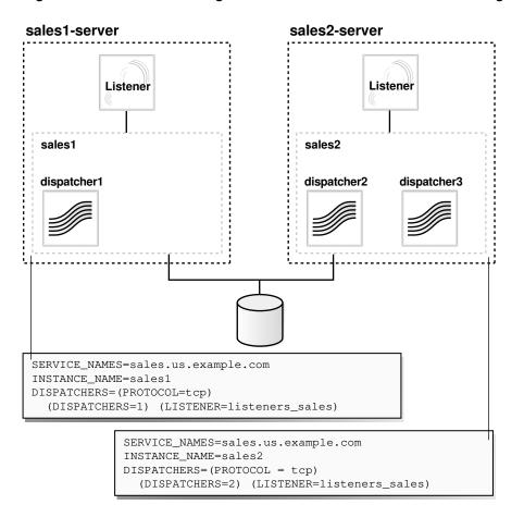
Figure 13-1 Load Balancing Environment for a Shared Server Configuration
