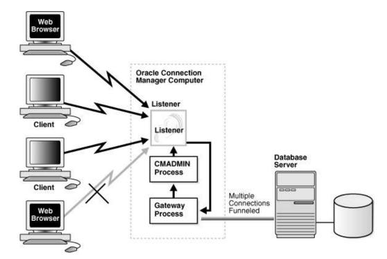
Figure 5-6 Oracle Connection Manager Architecture
