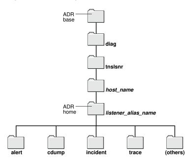
Figure 16-1 Directory Structure for an Oracle Net Listener Instance
