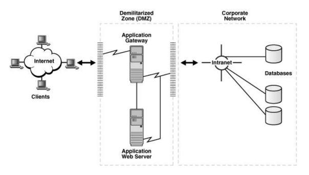
Figure 1-12 Internet Network Access Control with an Application Gateway
