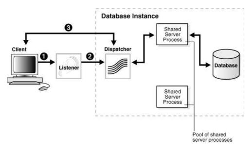
The following figure shows the role of a dispatcher in a redirected connection.
