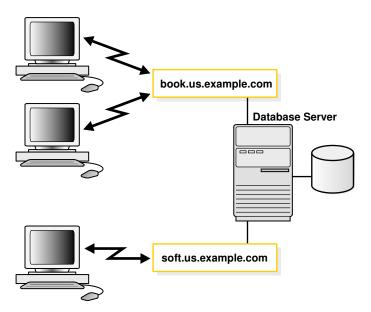
Figure 2-4 Multiple Services Associated with One Database
