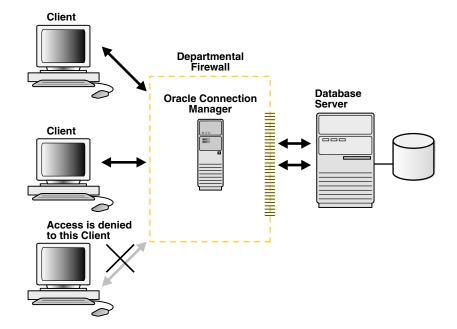
Figure 1-11 Intranet Network Access Control with Oracle Connection Manager
