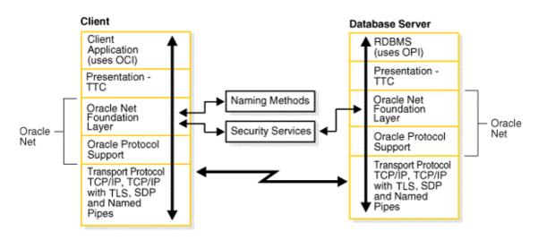
Figure 4-1 Layers Used in a Client/Server Application Connection
