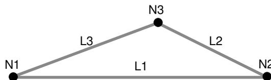
As shown in [Figure 5-6](#), link L1 is a straight line connecting nodes N1 and N2, link L2 is a straight line connecting nodes N2 and N3, and link L3 is a straight line connecting nodes N3 and N1. There are no other nodes on any of the links.
