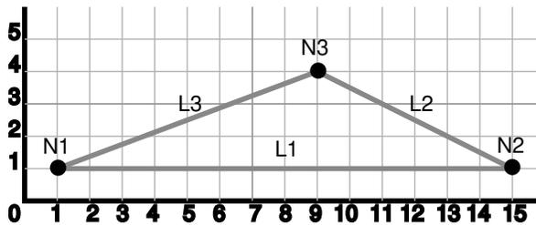
As shown in [Figure 5-5](#), node N1 is at point 1,1, node N2 is at point 15,1, and node N3 is at point 9,4. Link L1 is a straight line connecting nodes N1 and N2, link L2 is a straight line connecting nodes N2 and N3, and link L3 is a straight line connecting nodes N3 and N1. There are no other nodes or shape points on any of the links.
