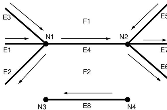
Table 1-2 shows the ID column values in the edge information table for edges E4 and E8 in Figure 1-6. (For clarity, Table 1-2 shows ID column values with alphabetical characters, such as E4 and N1; however, the ID columns actually contain numeric values only, specifically the numeric ID value associated with each named object.)
