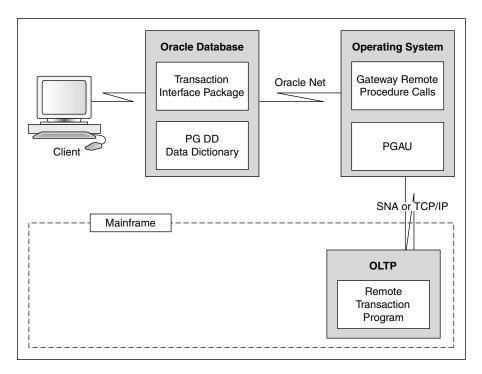
Figure 1-1 Relationship of Gateway and Oracle Database
