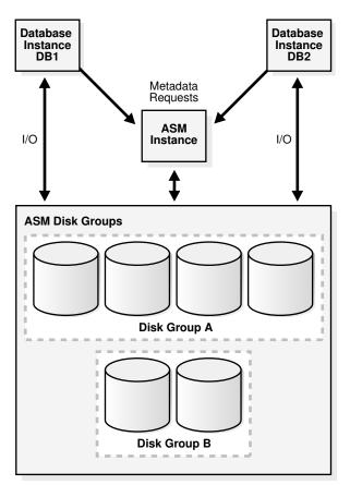
Figure 14-3 Oracle ASM Instance and Database Instances
