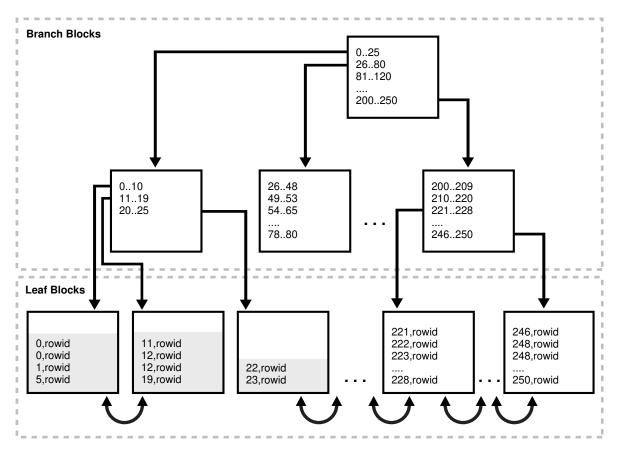
Figure 15-16 shows the index in Figure 15-15 after the index has been coalesced. The first two leaf blocks are now full, as indicated by the gray fill lines, and the third leaf block has been freed.
