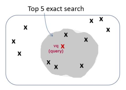
Depending on how your vector index was constructed, running a top-5 approximate similarity search in that context could return the five vectors shown on the third diagram. This is because the index creation process is using heuristics. So searching through the vector index may lead to different results compared to an exact search:
