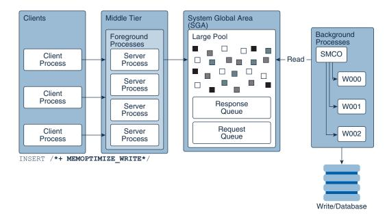
Figure 17-8 Deferred Insert Mechanism
