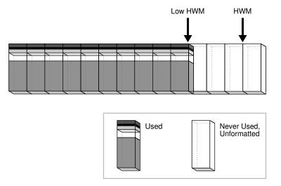
When the blocks between the HWM and low HWM are full, the HWM advances to the right and the low HWM advances to the location of the old HWM. As the database inserts data over time, the HWM continues to advance to the right, with the low HWM always trailing behind it. Unless you manually rebuild, truncate, or shrink the object, the HWM never retreats.
