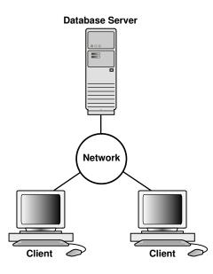
Figure 19-2 is a variation that depicts a distributed database. In this example, a database on one host accesses data on a separate database located on a different host.
