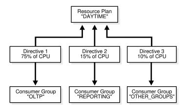
One problem that Resource Manager can solve is runaway queries, which can monitor using SQL Monitor. Resource Manager enables you to specify thresholds to identify and respond to runaway SQL statements. For example, you can specify thresholds for CPU time, elapsed time, physical or logical I/Os, and PGA usage by each foreground process in a consumer group. In response, Resource Manager can switch to a lower priority consumer group, terminate the SQL statement, or log the threshold violation.
