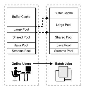
If you create a database with DBCA and choose the basic installation option, then Oracle Database enables automatic memory management by default.
