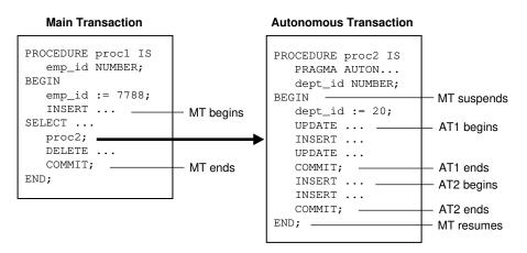
When you enter the executable section of an autonomous routine, the main routine suspends. When you exit the autonomous routine, the main routine resumes.
