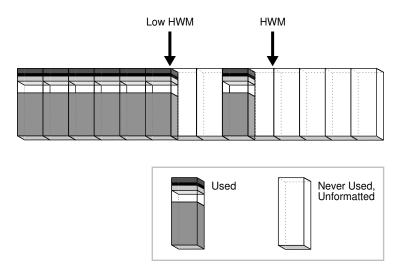
The low HWM is important in a full table scan. Because blocks below the HWM are formatted only when used, some blocks could be unformatted, as in Figure 15-26. For this reason, the database reads the bitmap block to obtain the location of the low HWM. The database reads all blocks up to the low HWM because they are known to be formatted, and then carefully reads only the formatted blocks between the low HWM and the HWM.
