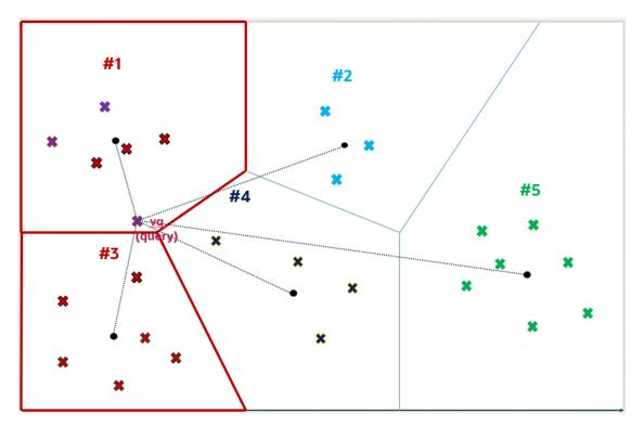
Once the  $\pm$  partitions are determined, they are fully scanned to identify, in this example, the top 5 nearest vectors. This number 5 can be different from k and you specify this number in your query. The five nearest vectors to vq found in partitions number 1 and 3 are highlighted in the following diagram.
