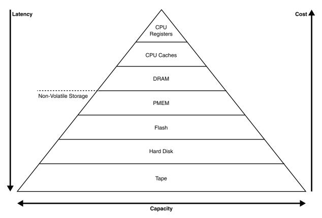
The database buffer cache resides in DRAM. Oracle processes have direct byte-addressable access to blocks in a PMEM filestore, which are mapped to the database buffer cache. The mapping mechanism is automatically invoked when you place a data file in a PMEM filestore.
