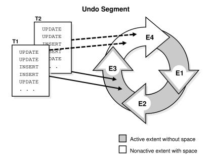
Figure 15-21 Ring of Allocated Extents in an Undo Segment
