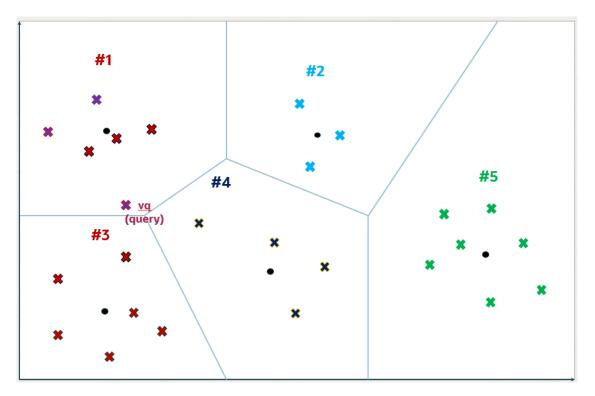
For a query vector vq, the search algorithm identifies the nearest i centroids, where i defaults to the square root of k but can be adjusted for a specific query by setting the NEIGHBOR PARTITION PROBES parameter. This adjustment allows for a trade-off between search speed and accuracy.
