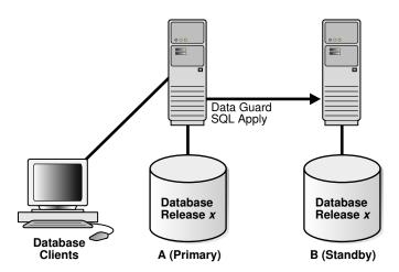
During the upgrade process, the Oracle Data Guard configuration operates with mixed database releases at several points in this process. Data protection is not available across releases. During these steps, consider having a second standby database in the Oracle Data Guard configuration to provide data protection.
