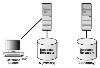
**3.** Restart SQL Apply and operate with release *x* on Database A and release *y* on Database B. To start SQL Apply, issue the following statement on Database B:
