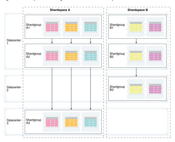
Figure 1-5 Composite Sharding With Oracle Data Guard Replication
