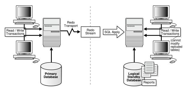
Figure 1-3 Automatic Updating of a Logical Standby Database
