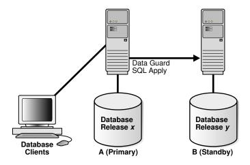
To monitor how quickly Database B is catching up to Database A, query the V\$LOGSTDBY PROGRESS view on Database B. For example:
