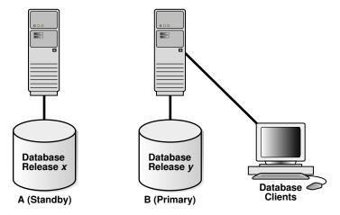
8. Database A is still running release *x* and cannot apply redo data from Database B until you upgrade it and start SQL Apply.
