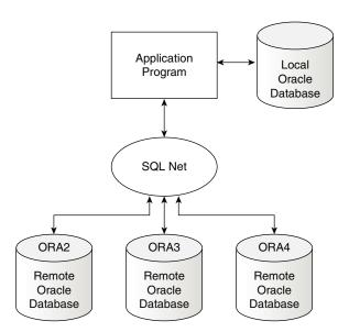
Figure 3-2 Connecting through SQL\*Net
