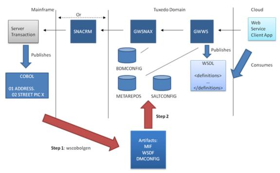
Figure 1-2 SOAP Inbound (Mainframe Transactions Exposed As A Web Service)
