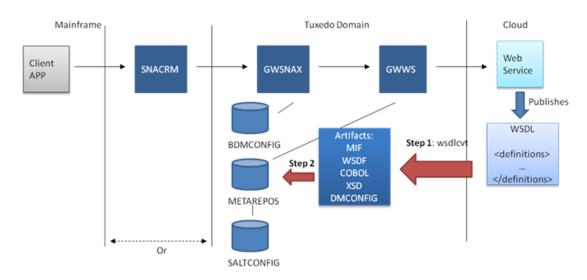
Figure 1-4 SOAP Outbound (Mainframe Invoking An External Web Service)
