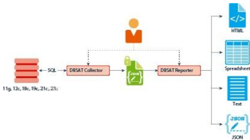
Figure Collector and Reporter Components and Architecture
