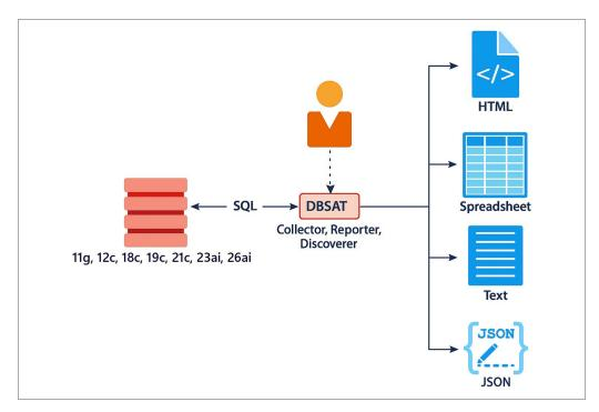
Figure 1-1 DBSAT Components, Sources, and Reports
