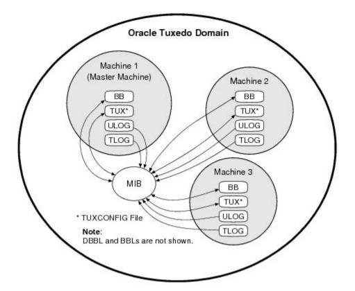
Figure 4-2 High-Level View of Oracle Tuxedo MIB Operation
