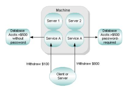
Figure 2-15 Data-Dependent Routing with Rule-Based Servers
