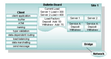
Figure 2-18 Load Balancing
