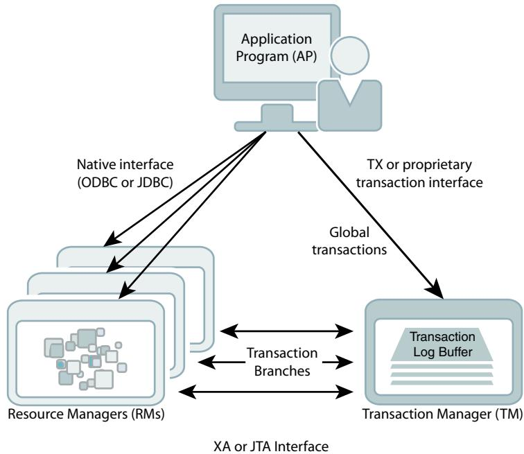
The TX interface is what applications use to communicate with a transaction manager. The figure shows an application communicating global transactions to the transaction manager. In the DTP model, the transaction manager breaks each global transaction down into multiple branches and distributes them to separate resource managers for service. It uses the JTA interface to coordinate each transaction branch with the appropriate resource manager.
