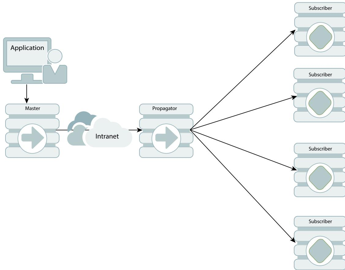
Propagators are also useful for distributing replication loads in configurations that involve a master database that must replicate to a large number of subscribers. For example, it is more efficient for the master to replicate to three propagators, rather than directly to the 12 subscribers as shown in [Figure 1-11](#).
