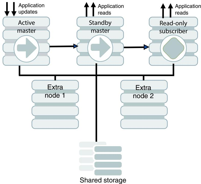
You can use Oracle Clusterware to start, monitor, and automatically fail over TimesTen databases and applications in response to node failures and other events. See [Clusterware Management](#) and [Recovering from Failures](#).
