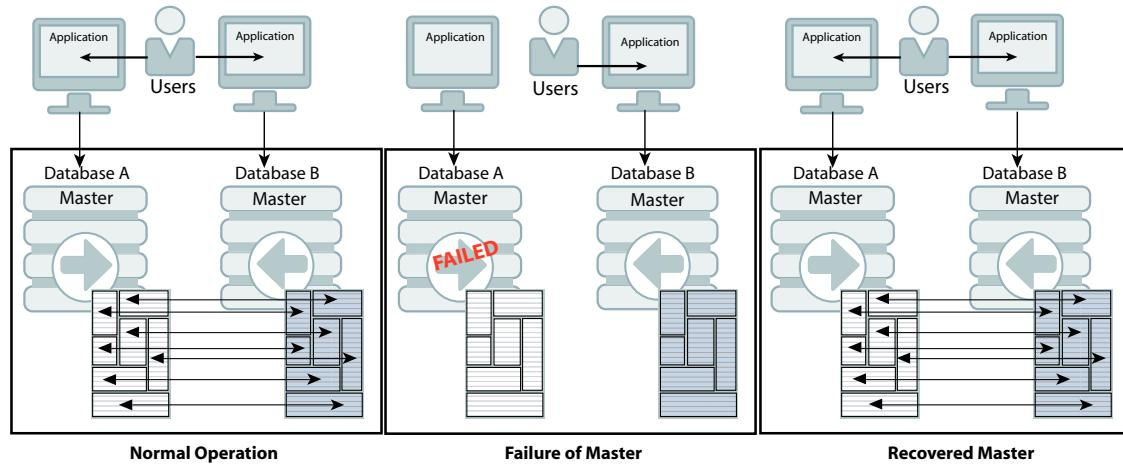
Similarly, the users in a split workload scheme must be shifted from the failed database to the surviving database. Because replication in a split workload scheme is not at the database level, you must use an `ALTER REPLICATION` statement to set a new master database. See [Replacing a Master Database in a Classic Replication Scheme](#). Upon recovery, the users can be moved back to the recovered master database.
