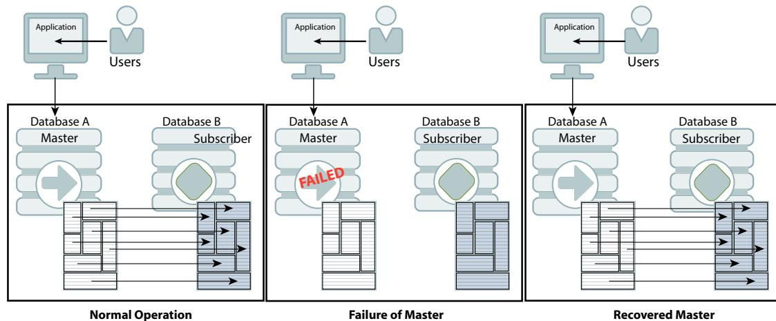
[Figure 9-2](#) shows a bidirectional distributed workload scheme in which the entire database is replicated. Failover in this type of classic replication scheme involves shifting the users of the application on the failed database to the application on the surviving database. Upon recovery, the workload can be redistributed to the application on the recovered database.
