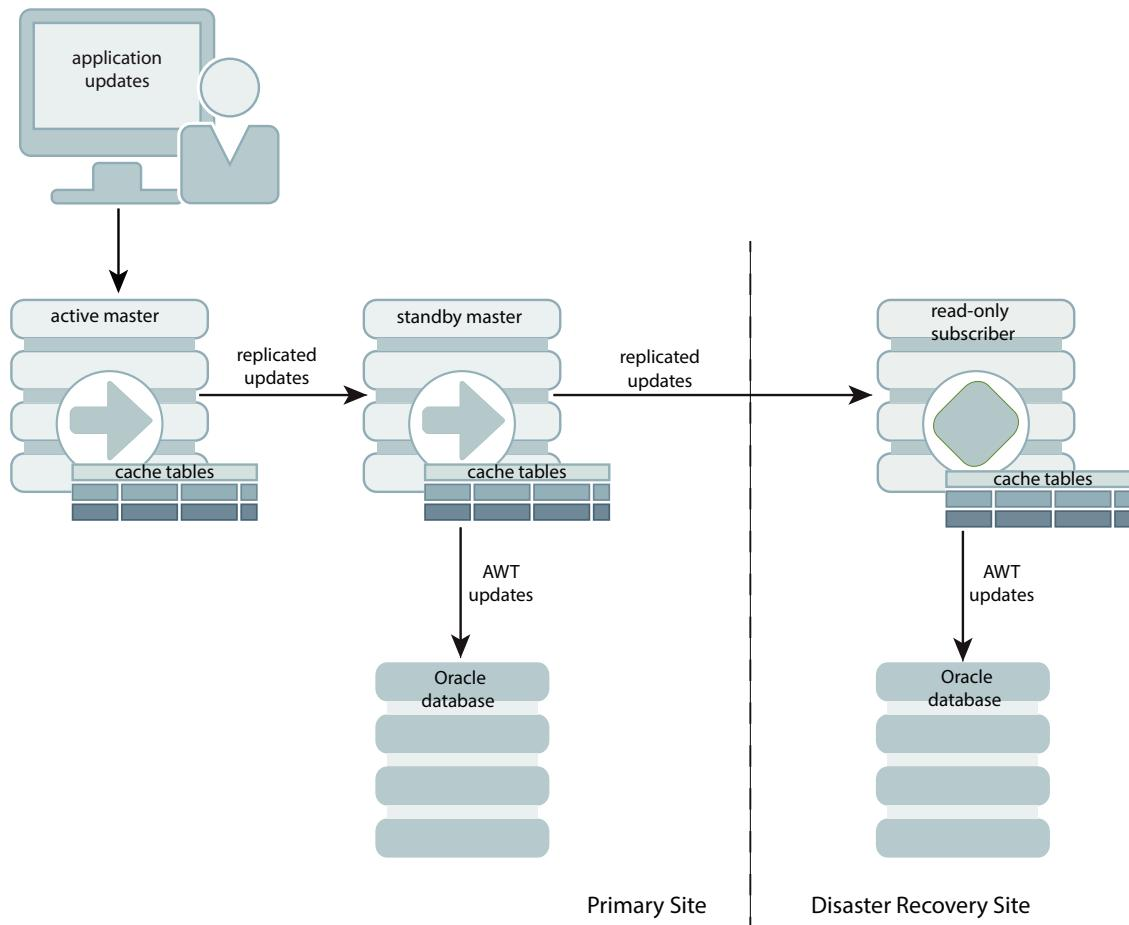
The standby database sends updates to cache group tables on the read-only subscriber. This special subscriber is located at a remote disaster recovery site and can propagate updates to a second Oracle database, also located at the disaster recovery site. You can set up more than one disaster recovery site with read-only subscribers and Oracle databases. See [Using a Disaster Recovery Subscriber in an Active Standby Pair](#).
