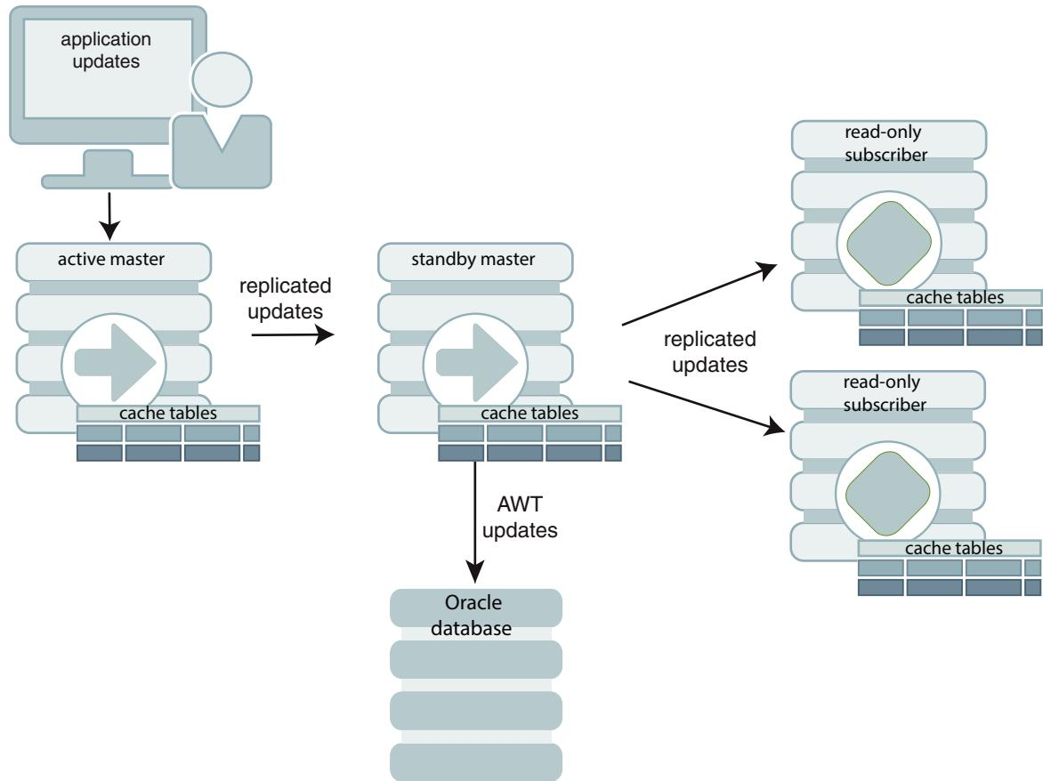
Application updates are made to the active database, the updates are replicated to the standby database, and then the updates are asynchronously written to the Oracle database by the standby. At the same time, the updates are also replicated from the standby to the read-only subscribers, which may be used to distribute the load from reading applications. The tables on the read-only subscribers are not in cache groups.
