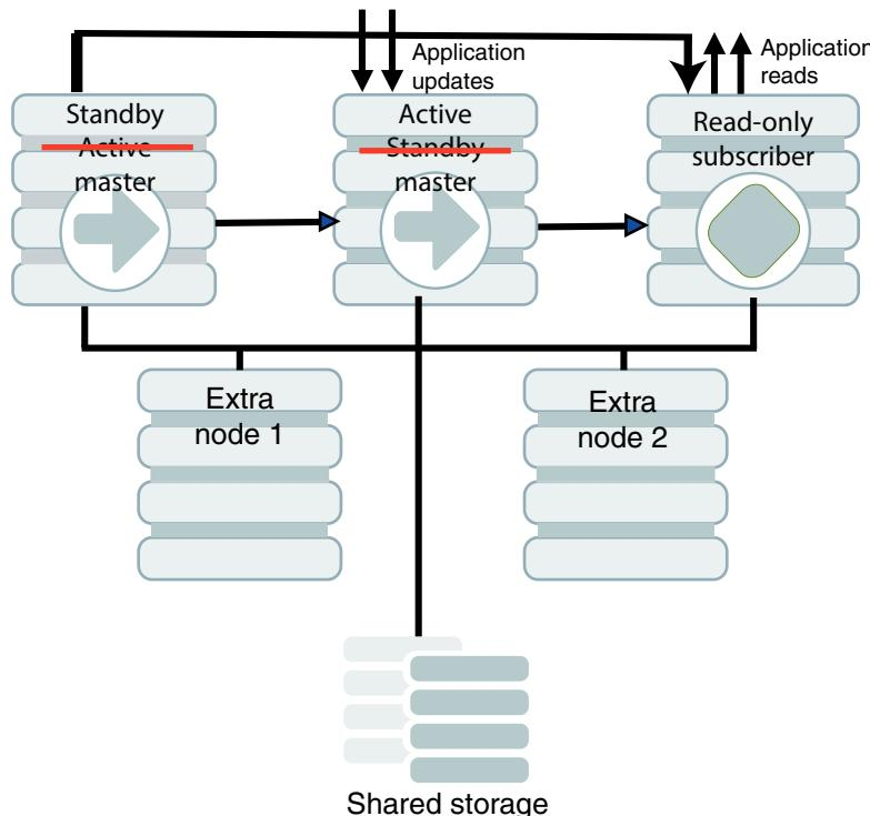
If the failure of the former active master is permanent and advanced availability is configured, Oracle Clusterware starts a standby master on one of the extra nodes.
