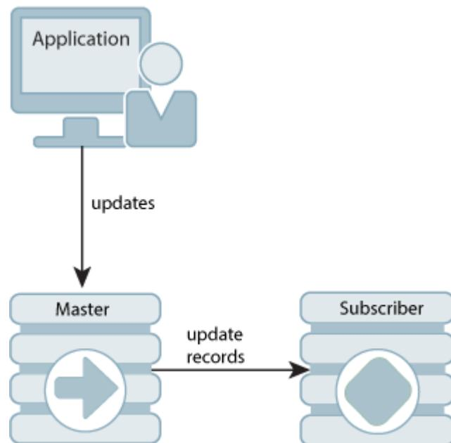
You can also configure your master and subscriber databases to selectively replicate some elements in a master database to subscribers. [Figure 1-6](#) shows examples of selective
