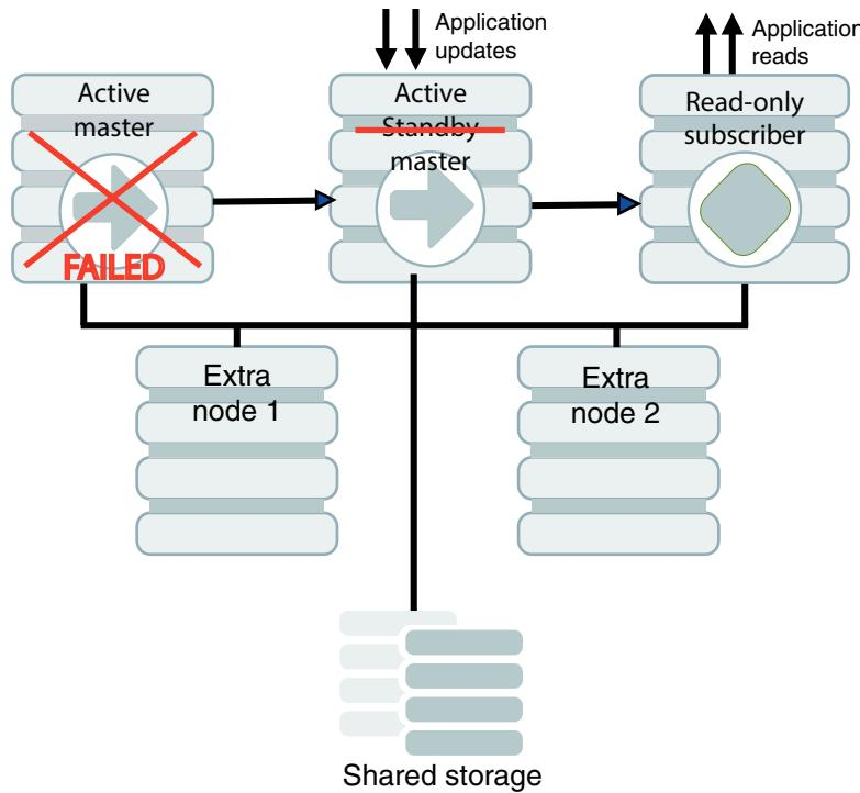
Oracle Clusterware tries to restart the database or host where the failure occurred. If it is successful, then that database becomes the standby database.
