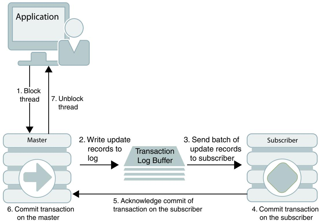
The following describes the replication behavior between a master and subscriber configured for return twosafe replication:
