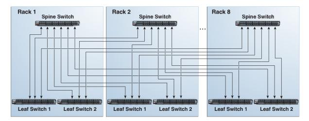
As shown in the preceding graphic, each leaf switch has eight inter-switch connections distributed over all spine switches. Each spine switch has 16 inter-switch connections distributed over all leaf switches. The leaf switches are not directly interconnected with other leaf switches, and the spine switches are not directly interconnected with the other spine switches.
