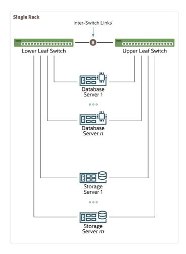
When connecting up to eight racks together, remove the eight existing inter-switch connections between each leaf switch on each rack. From each leaf switch, distribute eight connections over the spine switches in all racks. In multi-rack environments, the leaf switches inside a rack are no longer directly interconnected, as shown in the following graphic:
