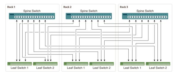
Figure 5-1 Connections Between Spine Switches and Leaf Switches for up to 8 Racks
