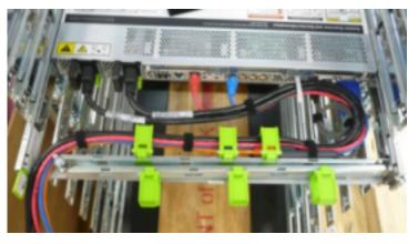
Route the cables through the CMA, and secure them with hook and loop straps at equal intervals.
