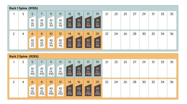
The following table describes the cable connections for the first spine switch (R1 SS) when cabling two racks together:
