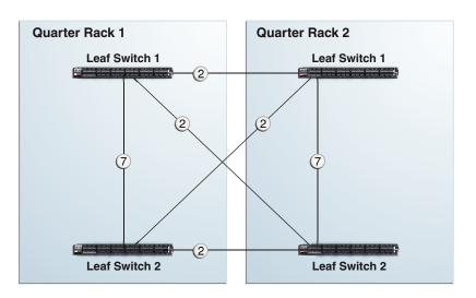
Figure 6-5 Leaf Switch Connections Between 2 Quarter Racks
