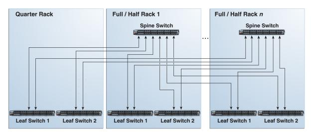
Figure 6-7 Leaf and Spine Switch Connections for a Quarter Rack Connected to One or More Half or Full Racks
