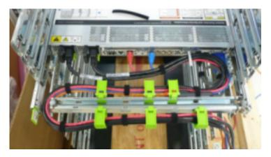
**8.** Connect the RDMA Network Fabric or TwinAx cables with the initial bend resting on the CMA. The TwinAx cables are for client access to the database servers.
