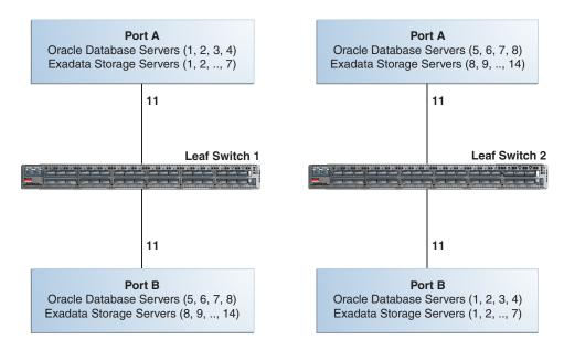
When connecting up to eight racks together, remove the seven existing inter-switch connections between each leaf switch, as well as the two connections between the leaf switches and the spine switch. From each leaf switch, distribute eight connections over the spine switches in all racks. In multi-rack environments, the leaf switches inside a rack are no longer directly interconnected, as shown in the following graphic:
