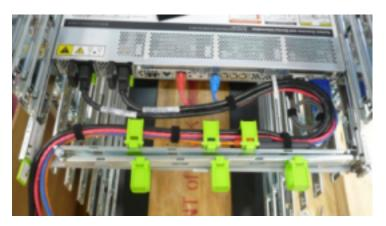
7. Route the cables through the CMA, and secure them with hook and loop straps at equal intervals.
