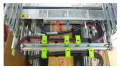
Secure the RDMA Network Fabric or TwinAx cables with hook and loop straps at equal intervals.
