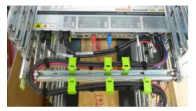
9. Secure the RDMA Network Fabric or TwinAx cables with hook and loop straps at equal intervals.
