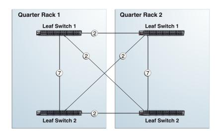
Figure 6-5 Leaf Switch Connections Between 2 Quarter Racks
