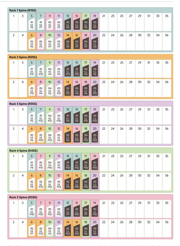
The following table describes the cable connections for the first spine switch (R1-SS) when cabling five racks together:
