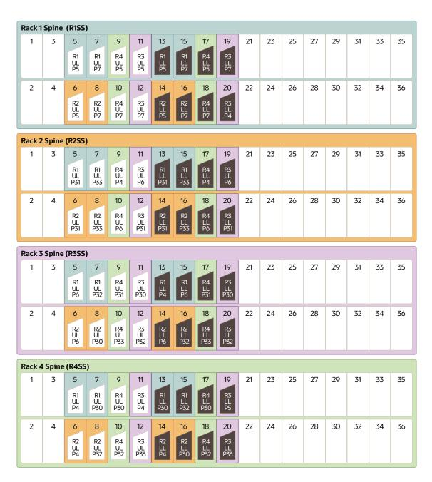
The following table describes the cable connections for the first spine switch (R1-SS) when cabling four racks together:
