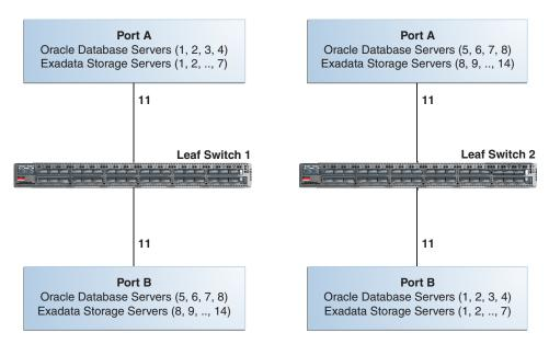
When connecting up to eight racks together, remove the seven existing inter-switch connections between each leaf switch, as well as the two connections between the leaf switches and the spine switch. From each leaf switch, distribute eight connections over the spine switches in all racks. In multi-rack environments, the leaf switches inside a rack are no longer directly interconnected, as shown in the following graphic:
