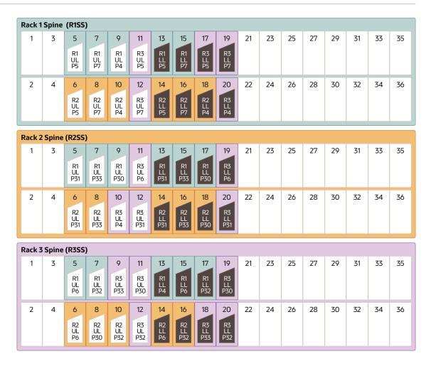
The following table describes the cable connections for the first spine switch (R1-SS) when cabling three racks together:
