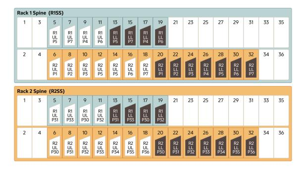
The following tables contain details for all of the RoCE Network Fabric cabling connections in a two-rack hybrid system with an X8M rack and a later model rack.
