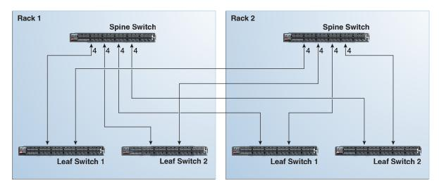
Figure 6-3 Connections Between Spine Switches and Leaf Switches Across Two Racks
