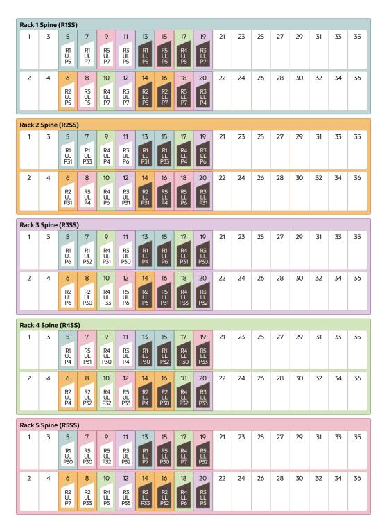
The following table describes the cable connections for the first spine switch (R1-SS) when cabling five racks together:
