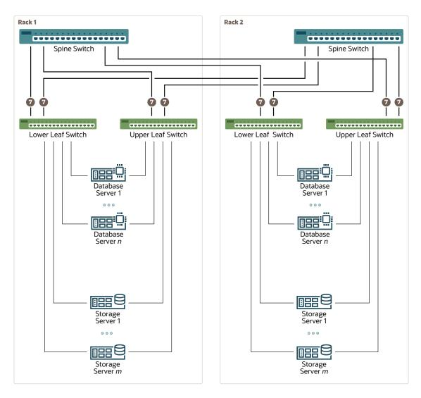
As shown in the preceding diagram, every leaf switch has 7 connections to every spine switch. The leaf switches are not directly interconnected with other leaf switches, and the spine switches are not directly interconnected with each other.
