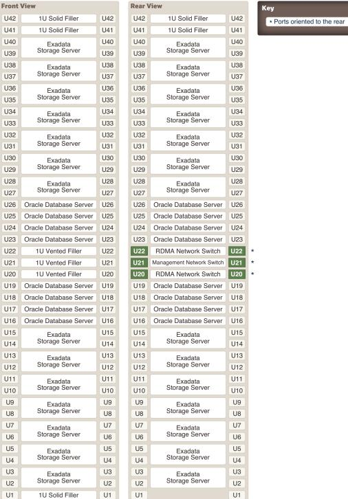
The following image shows the front and rear views of the component positioning in Oracle Exadata X8M-8.
