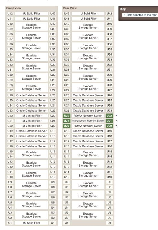
The following image shows the front and rear views of the component positioning in Oracle Exadata X9M-8.
