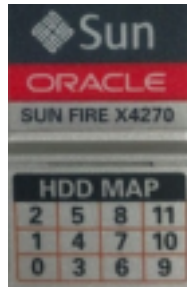
Figure 10-2 Disk Layout in Exadata Storage Server with Sun Fire X4270 M2 Servers
