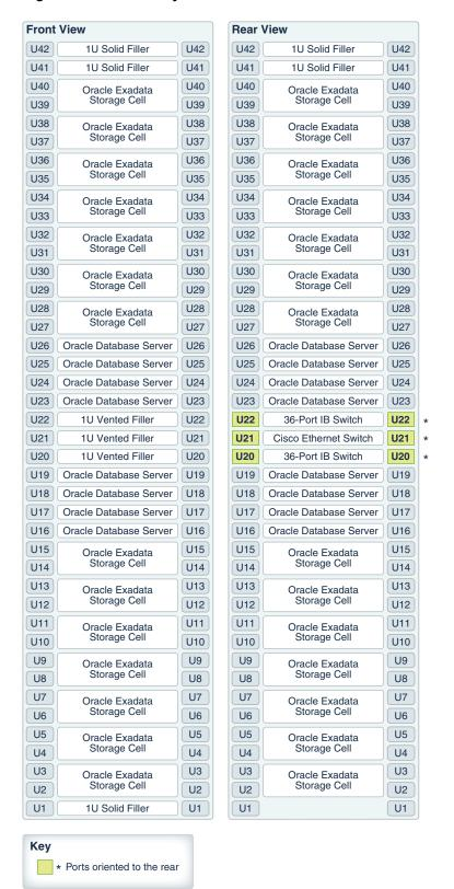
The following image shows the front and rear views of Oracle Exadata Database Machine X8-8 and X7-8.
