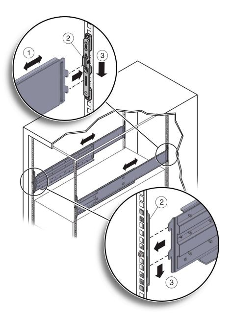
8. Thread the four M4  $\times$  10 flathead locking screws into the four adapter brackets [1]). These screws prevent the shelf rails from accidentally lifting out of the adapter
