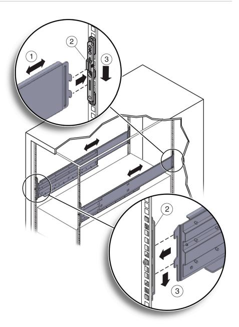
**8.** Thread the four M4 x 10 flathead locking screws into the four adapter brackets [1]). These screws prevent the shelf rails from accidentally lifting out of the adapter brackets. The following figure shows how to install the lock screws to the adapter
