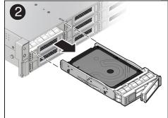
4. Align the replacement drive with the drive slot.
