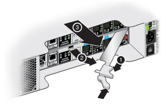
3. Open the lever in the new I/O module if it is not already open.
