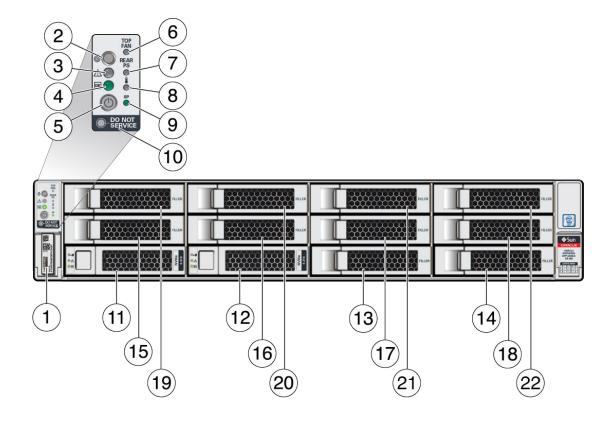
The following figure shows the components on the front panel of an **Oracle Database Appliance X8-2M**.
