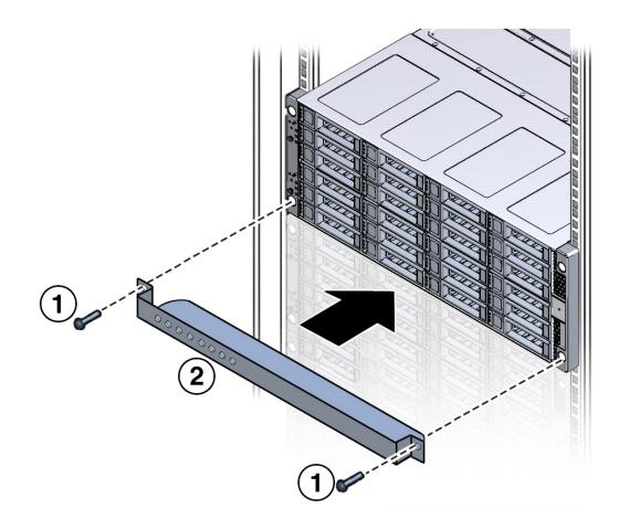
Use the two long screws (either the M6 x 30 mm screws or the 10-32 x 1.25 inch screws)
