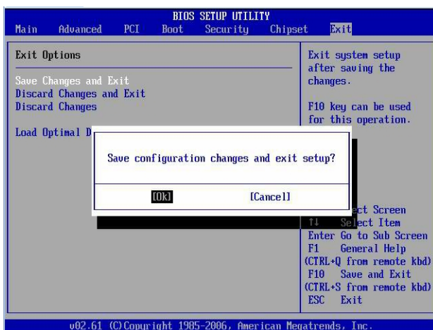
Figure A-2 BIOS Setup Utility Save and Exit Screen
