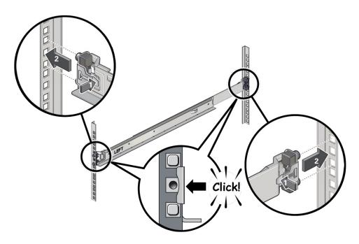
d. Close the rail clamps over the rails by releasing the clamp lever.
