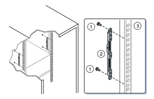
The following figure shows the rear adapter brackets being attached to a square-hole rack:
