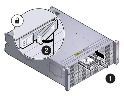
Once installed, the system should automatically detect and use the replacement drive. Ensure that the green OK indicator for the replacement drive lights to show that the drive is ready.
